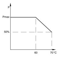
For UL and CSA the maximum temperature is 60°C (70°C for the 20 A model)
