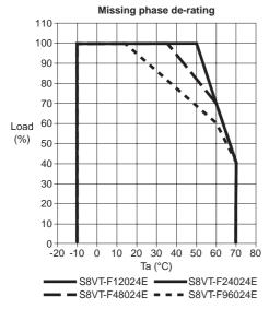
**Note:** In two phase operation, the specification for EMC performance, hold-up time, efficiency and output ripple will no longer be valid.
